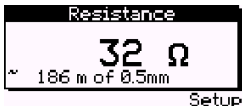
Figure 3 Aurora Presto DMM Typical Tip - Ring Isolation Measurement
