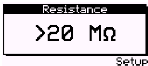
Aurora Presto DMM Typical Isolation Resistance Measurement
