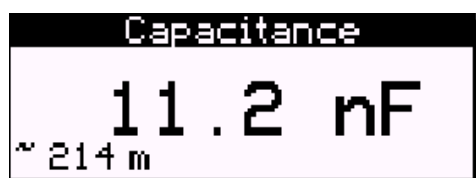
Figure 5 Typical Aurora Presto Screen Shot of Capacitance With Distance Approximation
