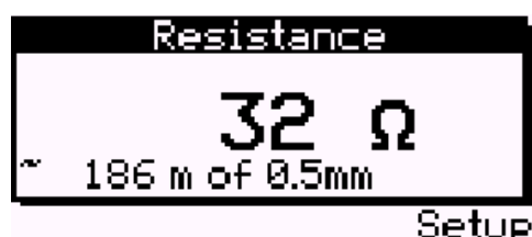
Figure 6 Typical Aurora Presto Screen Shot of Resistance With Distance Approximation
