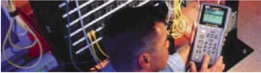
Figure 1.12 LANTEK 7 cable tester compliant with Categories 3/5e/6 and 7/ISO F standards, with a frequency range up to 750 MHz.
