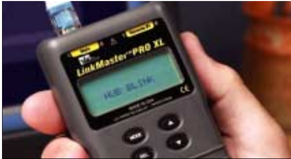
Figure 1.2 LinkMaster, a wiremap tester suitable for Cat 5 verification all four twisted pair.
